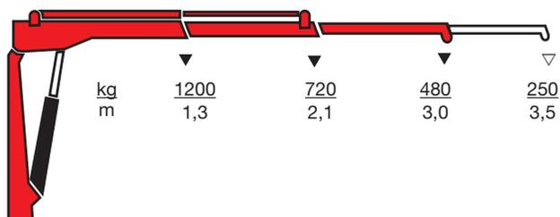
▼ Lifting capacity without manual extensions
