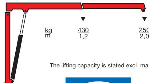
The lifting capacity is stated excl. manual extensions
